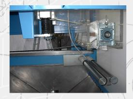
Over the years, **AIGLE** has developed several **Flocking Equipment for Rubber Sleeves**: they are tubular sheaths with different diameters and lengths that are flocked and then vulcanized; subsequently they are cut into strips in a closed loop so that they can be used as transmission belts for engines.
