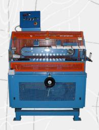
The **Caterpillar mod. CTP800** consists of a strong, motorized frame installed in the lower part, and a couple of opposed 10 mm rubber covered "Poly V" belts, installed in the upper part.
