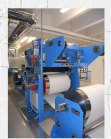
The Laminating Group mod. GRA/1 is for wet lamination and dry-coat lamination technology. It consists of:
