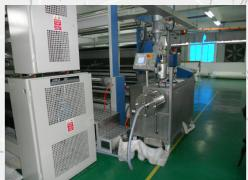
The Coating Machine mod. BSR/F is used to coat fabric (with resin and/or adhesives).
