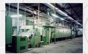
Heating system, which is equipped with a recirculation fan, an oil battery, blowing channels, an air recovery channel and a filter. To ensure uniform heating and air distribution, fields are opposed on the left and the right side.
