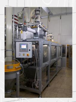
The Suction & Pre-Cleaning Group mod. PRCP and mod. Jet-Matic is placed after the flocking machine to ensure a good pre-cleaning of the profile prior to its entrance in the oven and also to avoid excessive dispersion of flock during the various working phases.
