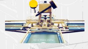
The Manual Flocking Device mod. EASY FLOCK/N is a flocking unit for samples and limited/batch productions.
