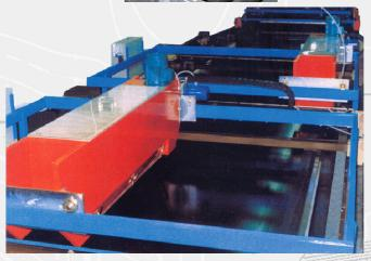
The system is composed of one or more **Flocking Units** that can be mounted on the stations of any flat screen printing line.
